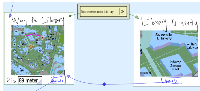
(a) Design #1 shows the entire campus and a detailed map is automatically shown when a user gets close to a target. Here the scenario “Bob moves near library” triggers showing a detailed map around the library.
