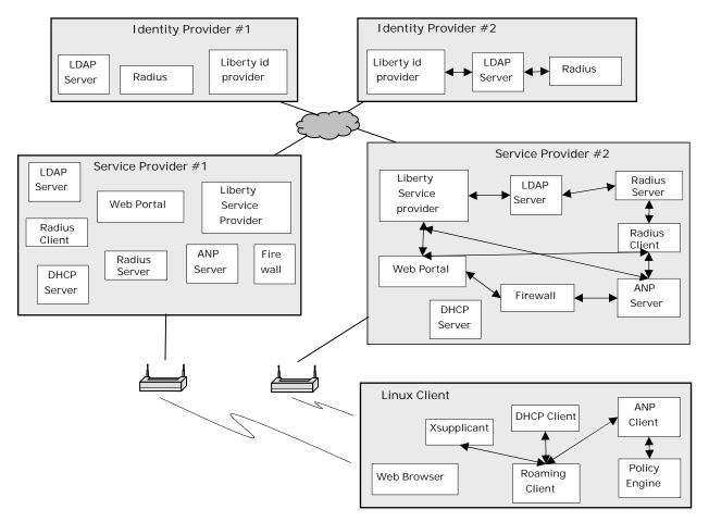
Figure 24: Testbed Software Components
