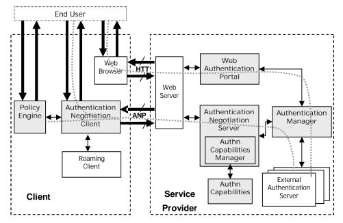
**Figure 5: Authentication Flow Adaptation Architecture**
