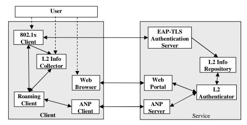
Figure 21: Compound Link Layer – Web Based Authentication Architecture
