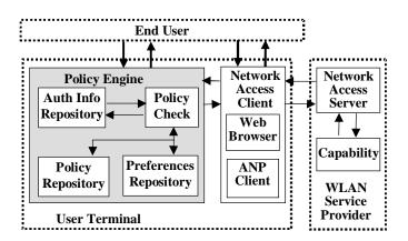
Figure 15: Policy Engine Block Diagram
