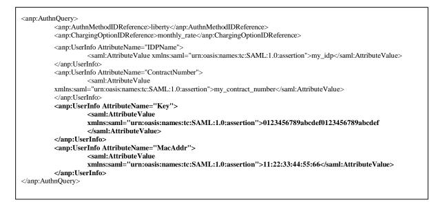
Figure 20: Authentication Query Example with Link Layer Information
