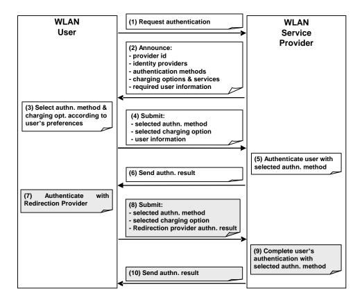
**Figure 4: Authentication Flow Adaptation Sequence**
