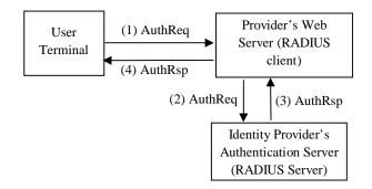
**Figure 2: Proxy-based RADIUS Authentication**
