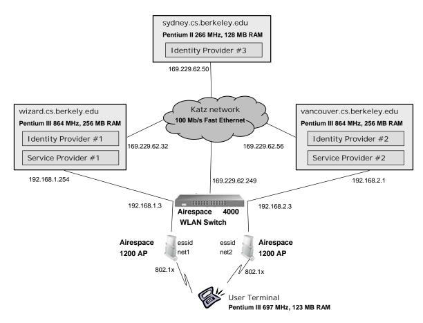
Figure 23: Testbed Physical Layout
