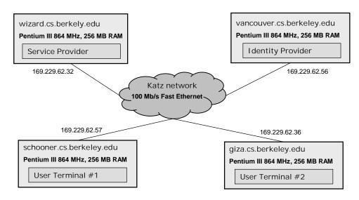
Figure 27: Load Testbed
