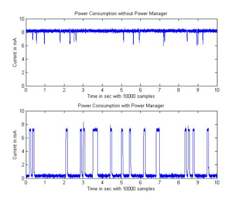
Figure 5-1: Measured Current at an Intermediate Node
