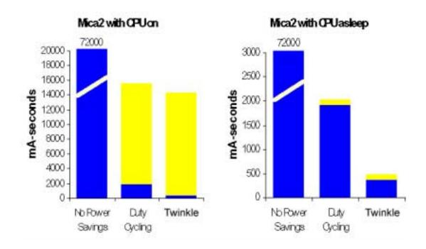
Figure 7-5: Mica2 Estimate (mA-seconds)
