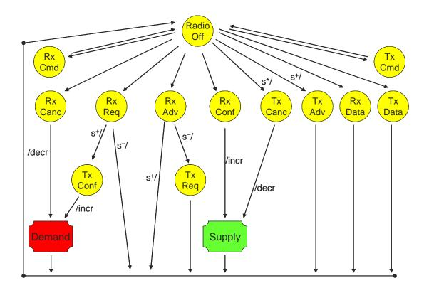
Figure 3-7: FPS State Diagram
