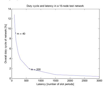
**Figure 5-6: Duty Cycle vs Latency**
