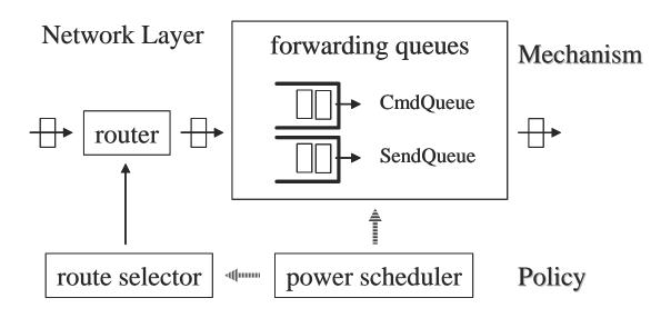
Figure 8-1: Separating Policy from Mechanism
