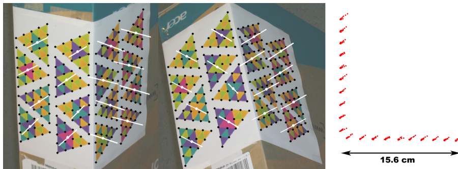
Figure 4: We demonstrate the ability to obtain a metric reconstruction from two orthographic views of a textured scene. We paste a triangle pattern on a box, forming two sections at a roughly 90 degree angle. Using both points and normals, we reconstruct the point locations by computing an orthographic camera calibration. Our calibration error is on average 2.41 pixels and 1.74 degrees. (photos taken with a consumer camera at maximum zoom to approximate orthography) To evaluate the results, we fit two planes to the two point sets and compute the angle between the planes to be 90.67 degrees (we estimate 90 degrees from world geometry). When fitting the plane the MSE distance from the points to the plane is 2.57 pixels or 1.69 mm. The physical paper isn't completely flat — deviations of 2mm appear physically plausible.
