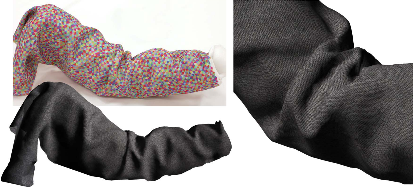
Figure 1: High resolution meshes of cloth can be captured from multiple images of an actual piece of cloth. We print a pattern on the cloth that uses an unlimited number of colors to build a set of features that can be easily recognized in challenging conditions, such as the folds in the elbow of this figure. The folds in the crease of the elbow on the right are the shape of actual folds in real cloth at a level of detail that is not easily simulated. This reconstructed mesh is made of 7,557 vertices comprising 15,036 triangles and has a reprojection error (a measure of the alignment between the model and image data) of 0.23 mm (230 \mu\text{m} ) or 0.05% of the object size.
