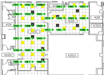
Fig. 3. 28 mote Omega Testbed at UC Berkeley
