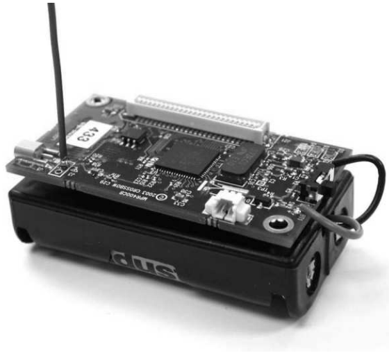
Figure 4.13: Mica2 sensors used for location sensor client.
