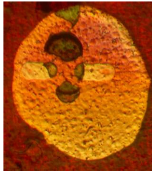
Figure 5.5: Discontinuous semiconductor film resulting from thick electrodes and “pooling” of drops.
