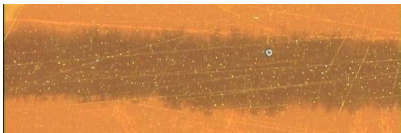
Figure 8.3: Ink IV, group B ink, forms a continuous film, but the edges are deformed and there is a high degree of spreading.
