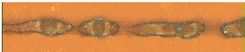
Figure 8.4: Gravure printed \alpha -terpineol ink showing the distortion that occurs before drying.
