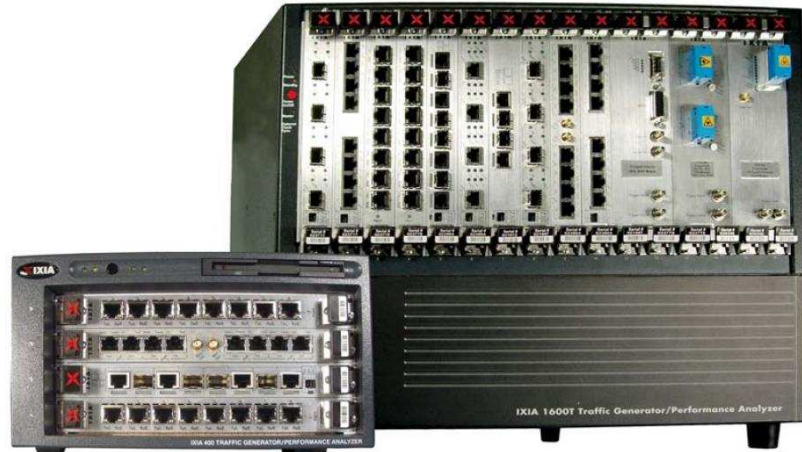
Figure 3.3. The active packet injection device, the IXIA 400T (left) that we used. (Courtesy: IXIA [Ixi])
