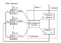
Figure 2: Our in-network tracking and detection framework.
