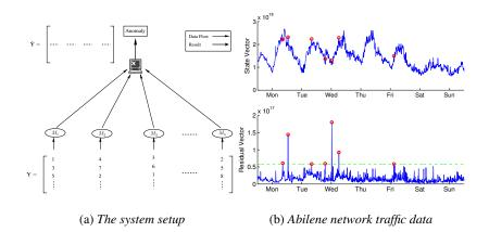
Figure 1: (a) The distributed monitoring system; (b) Data sample  $(||\mathbf{y}||^2)$  collected over one week (top); its projection in residual subspace (bottom). Dashed line represents a threshold for anomaly detection.
