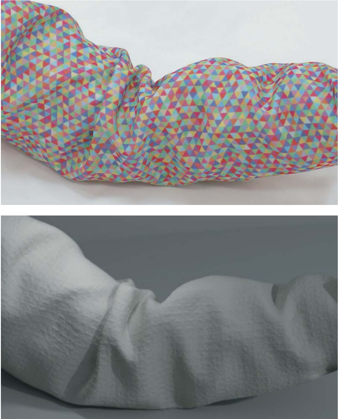
Figure 6.5: We reconstruct the shape of a static arm using thousands of markers to estimate the geometry.
