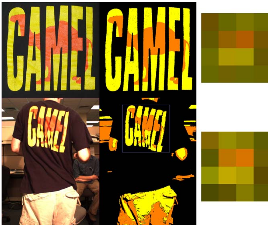
Figure 2.5: Our method requires a frontal view of the texture ( top row ) and a target image ( bottom row ). We quantize the colors using a color classifier, then compute a 4 \times 4 color histogram, with separate bins for each color channel. In this case, with three colors (black, orange and yellow), our descriptor is 4 \times 4 \times 3 . We visualize this descriptor by reconstructing the colors and normalizing appropriately ( right ). A search for the descriptor in a subsampled version of the target image reveals the closest match ( bottom right ).
