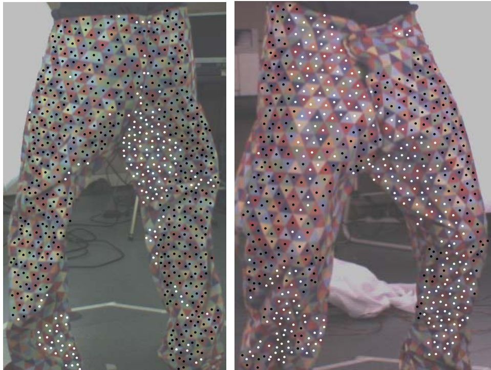
Figure 7.13: With only six cameras, it is common for points to be seen in only one view. We can still use these points for reconstruction by confining the point to a ray and using volume and strain constraints (section 7.5). In the images above, black points are detected in at least two cameras while white points are viewed in only one camera. Notice that the colors in these two images are significantly different: they were taken using the same model cameras with identical settings at the same moment in time, yet the internal processing of the cameras yields different colors.
