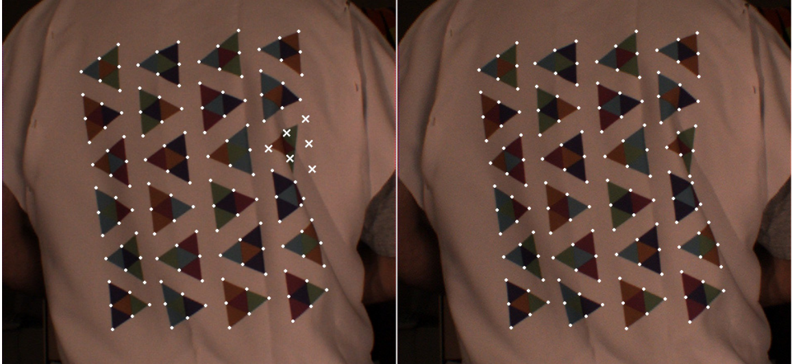
Figure 2.3: Here we see one of the problems with a top down method for marker identification: large regions go missing with small changes in geometry. On the left a single triangle is not detected. In this case, we interpolate the location of the triangle using a linear estimate based on the locations of the other triangles (shown as white Xs). In the next frame ( right ), the corresponding triangle is detected with a substantially different position — causing a pop in the video sequence.
