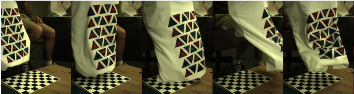
Figure 7.6: Above is a selection of images taken from a single camera — the cloth moves significantly during different parts of the sequence. A planar calibration pattern (checkerboard) allows us to compare calibration methods (checkerboard calibration performed using code from [Bouguet 05]). We calibrate over time using several frames in order to cover the space well. Figure 7.7 shows calibration results for this sequence.
