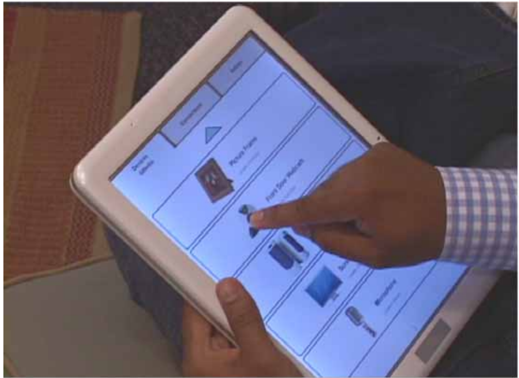
Figure 5-1: OSCAR is a handheld, touchscreen based application that allows users to discover, connect, and control multiple devices and services on a home network, as well as create re-usable compositions for quick access to commonly-used functions.
