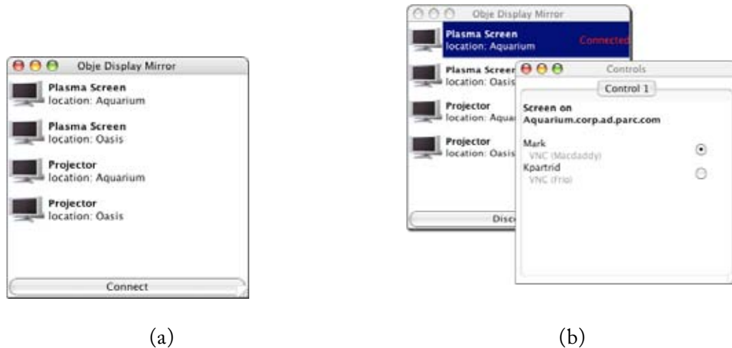
Figure 4-4: The Display Mirror client before and after a connection is made. First, (a) the user sees a list of available screens. After connection, a control UI (b) is presented to all connected users of the selected screen, allowing control of the display to be shared.
