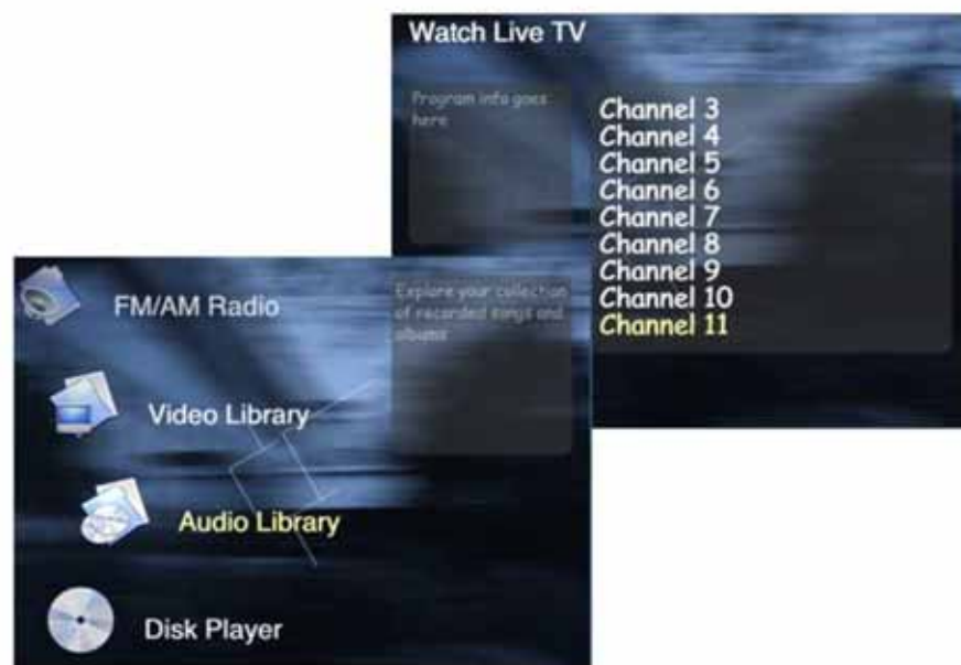
Figure 3-8: Two main screens from the Objé set-top application. The image on the lower left shows some of the main menu items in the user interface. Each selection represents a built in template of functionality related to a particular media or device type. The image on the upper right shows a specific user interface for tuning channels on a television tuner component.
