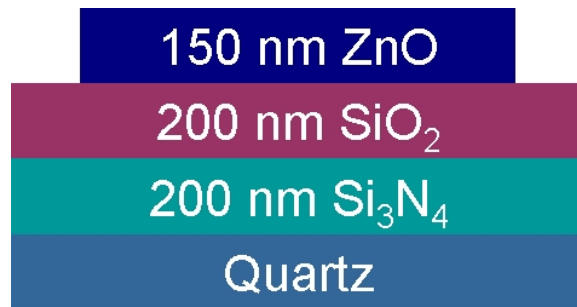
Figure 5.25. Structure of the Hall Effect samples.
