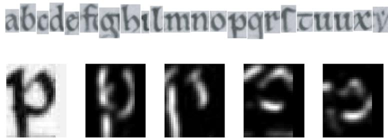
Figure 3.4: **Top**, the 22 instances, one per letter, used to train our emission model. These templates are extracted by hand from the Terence document. **Bottom**, the five image channels for a single letter.
