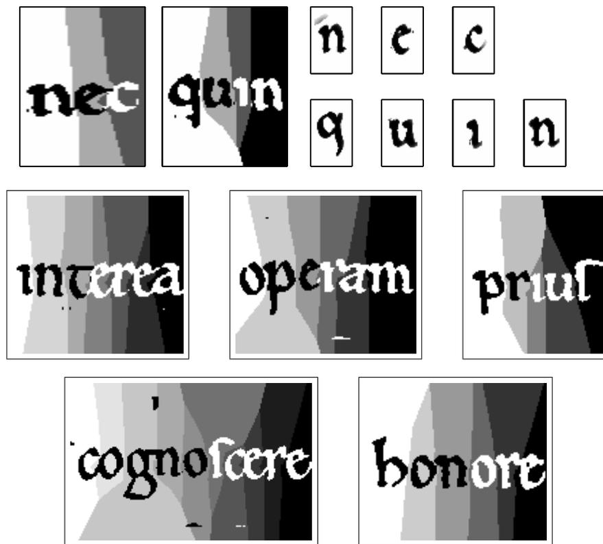
Figure 4.5: **Extracting Templates** For a region with sufficiently high confidence margin, we construct the maximum likelihood template from our current exemplars. top left, and we assign pixels from the original image to a template based on its distance to the nearest pixel in the template image, extracting new glyph exemplars top right. These new glyphs become the exemplars for our next round of training. Lines 2 and 3 show additional template masks from high confidence regions.
