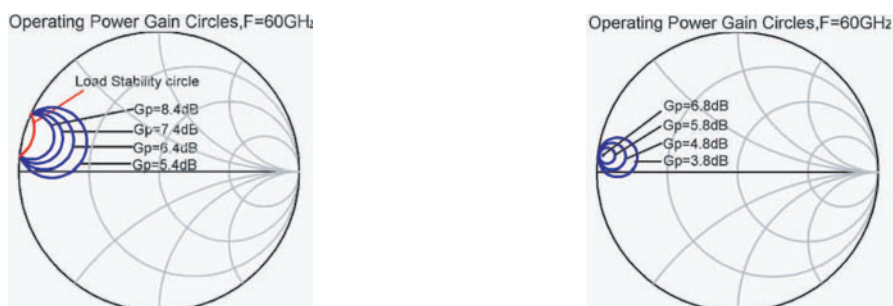
Figure 3.9: Load impedance contours of constant device power gain and contours of constant output power.
