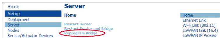
Figure 1.3: Reprogramming the bridge node
