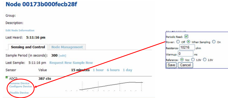
Figure 1.24: Configure ADC port, resistor, reference
