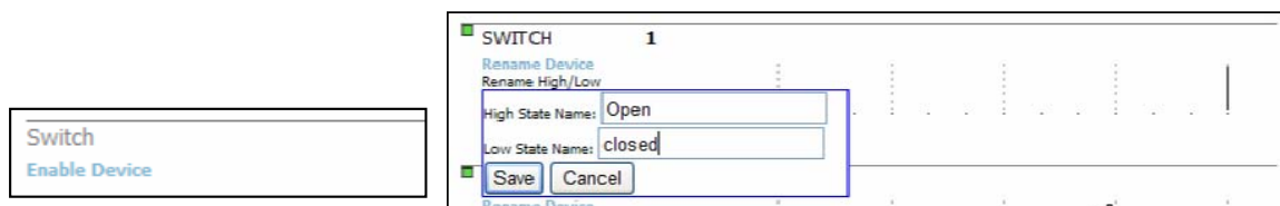
Figure 1.20: Configuring switch port: (a) enable device, (b) name the states
