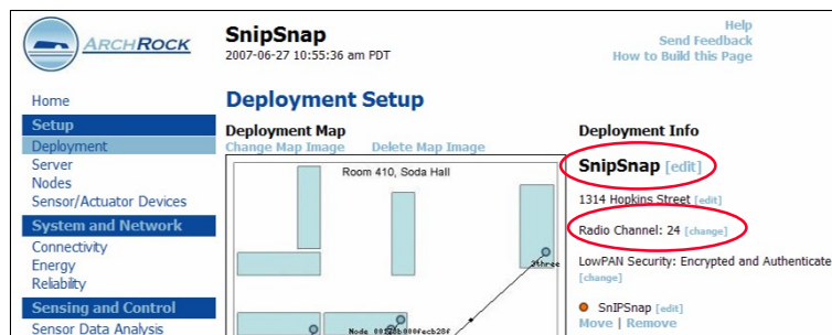
Figure 1.2: Setting up the 802.15.4 radio channel for each group
