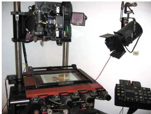
Figure 3-10: Animation stand used by animator 2. This facilitates lighting and moving of animation cels during final photography.
