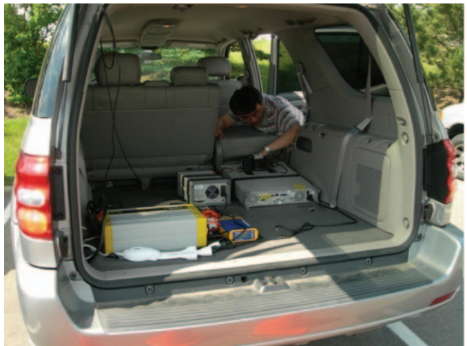
Fig. 2. Channel sounding transmitter vehicular setup.
