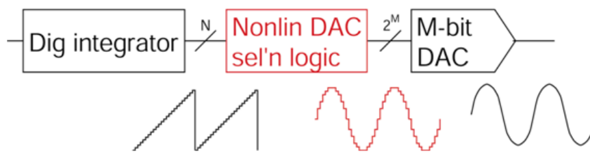
Figure 4.13: DDFS architecture with trigonometric function embedded in DAC selection logic
