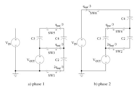
Figure 4: Switch charge flows
