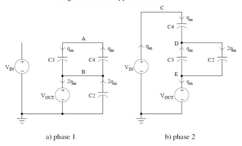
Figure 3: Capacitor charge flows
