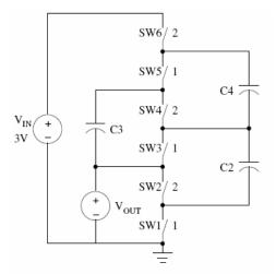
Figure 2: Ladder-type SC converter
