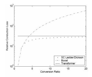
Figure 1: Conduction Loss Comparison
