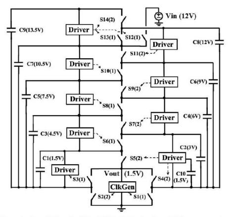
Figure 9. Overall Circuit of the 12V-to-1.5V step down Dickson converter. The numbers in bracket of the switches indicate their respective clock phases. The dotted arrows show the respective driver block that drives each powertrain switch
