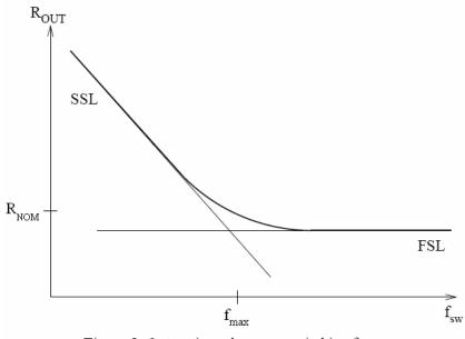
Figure 5: Output impedance vs. switching frequency
