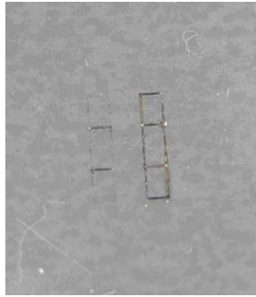
Figure A.4: Damage from laser cutting with large window size (right) compared with small window size (left, difficult to even see)
