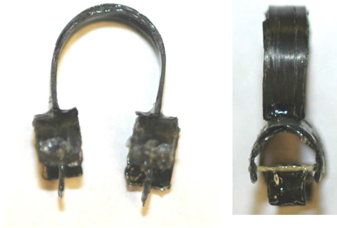
Figure 3.8: Front and side view of carbon fiber dynamometer spring.
