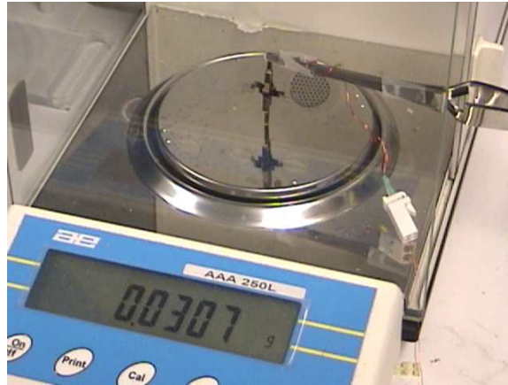
Figure 5.24: Lift test setup of MFI revision 2.
