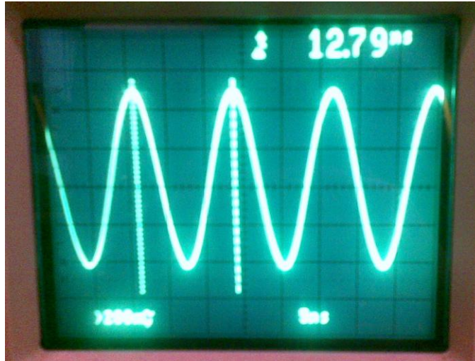
Fig. 7. Snapshot of the oscilloscope screen showing the signal generated by a 1 \mu\text{m} gate ring oscillator
