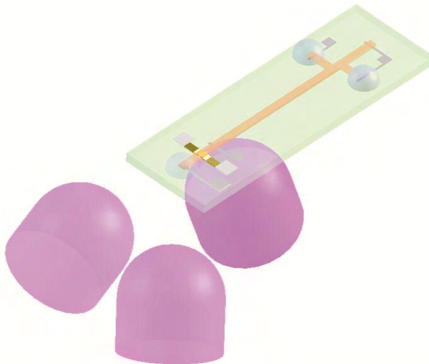
Figure 4.2: Model of the optical setup for the PNTFT sensor integrated into the IPSMS.
