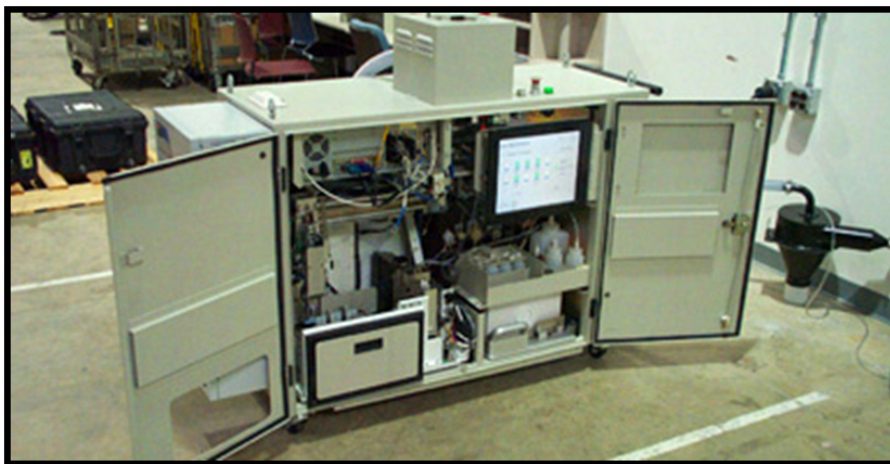
Figure 1.2: Real-time Polymerase Chain Reaction (PCR) analysis system built by Cepheid, Inc.
