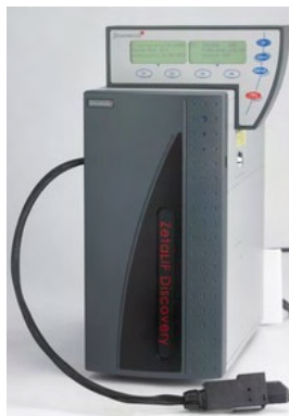
Figure 1.7: Compact laser-induced fluorescence detector made by Picometrics, Inc. [4]
