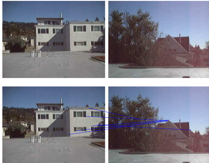
Figure 2.2: (Top Row) Images from two wide baseline cameras and it is difficult to tell how the cameras' fields of view are related. (Bottom Row) Images from the same two cameras with SIFT features applied and the matching shown. The matching is incorrect as the static features in each image are not the same.
