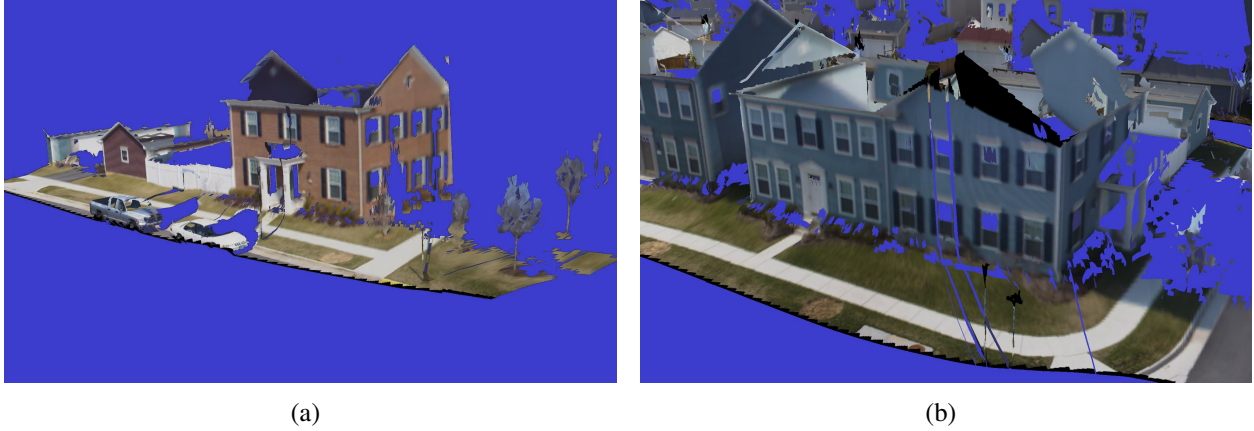
Figure 7: Surface reconstruction result from S1. (a) The entire 3D surface model of point cloud 1. (b) A portion of the 3D surface model of point cloud 2.
