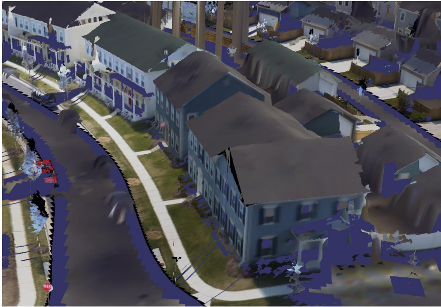
Figure 13: Combined terrestrial and airborne mesh of a portion of point cloud 2. For details on the ground-air merge, please see [2].
