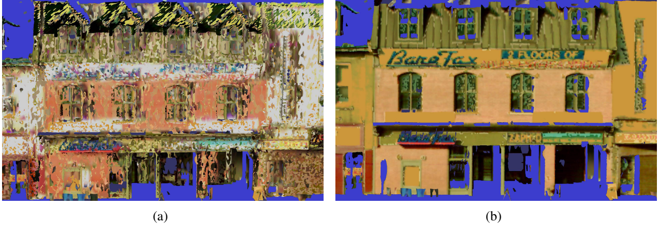
Figure 10: Mesh (a) with redundant surfaces and (b) without redundant surfaces. The point clouds used to generate these meshes are not from S1 or S2. Instead, they are from a dataset which was obtained using multiple sensor passes.
