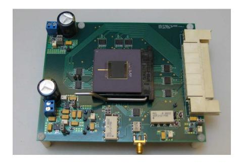
Figure 5.16: Printed circuit board hosting the packaged chip.
