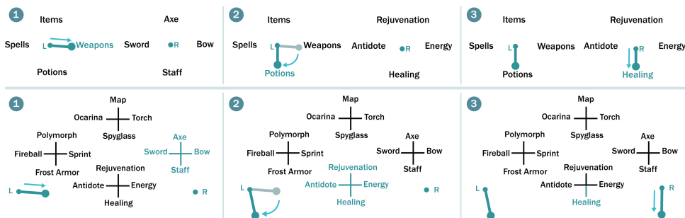
Fig. 16. Top: Hierarchical Display - The left hand explores the parent menu items by dragging through menu items, and the child menu items continuously update for the right hand. Bottom: Full-Breadth Display - The entire menu space is displayed, and the left hand chooses the four-item cluster, while the right hand chooses the item within a cluster.
