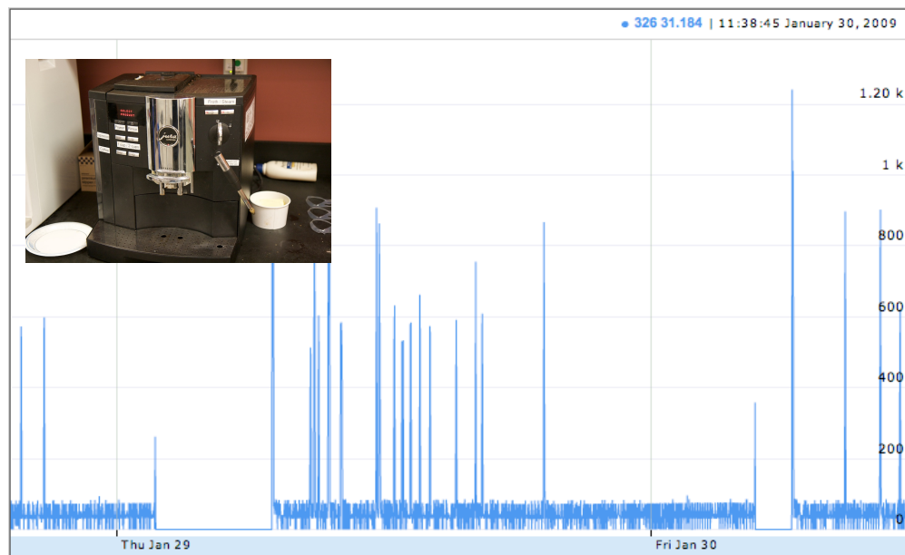
Figure 4.7: Power trace of a coffee maker shows that ACme-A is able to measure appliances with high power pulses.
