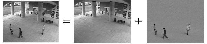
Figure 11: Sample output of Robust PCA for stationary video background subtraction
