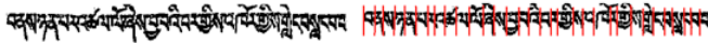
Fig. 12. A line of Tibetan block print, the red lines corresponds to the segmentation points.
