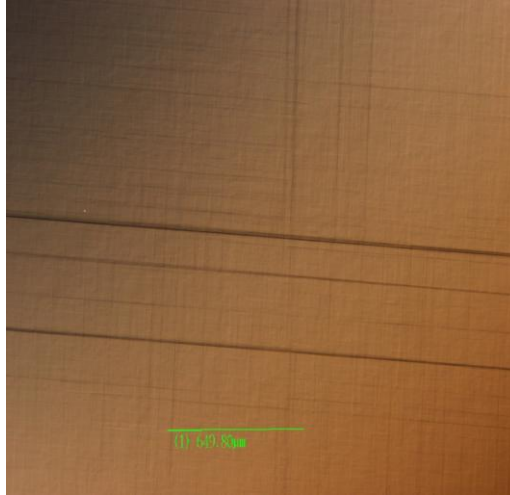
Figure 6.3 Slip lines seen visually across the entire wafer except at the center of the wafer.
