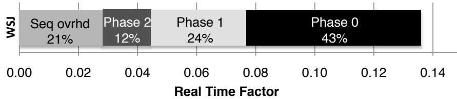
Figure 6.1: The recognition speed shown as real time factor (RTF) demonstrated with the Wall Street Journal corpus at 8.0% WER
