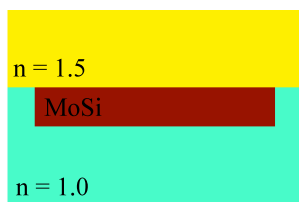
(a) MoSi mask blank with refractive index 2.343 + 0.586j and 77.2 nm thick
