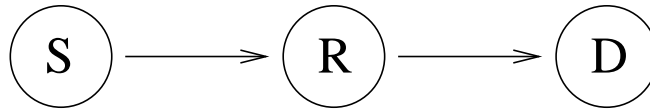
Figure 4.2: This simple network illustrates the starvation problem that can occur when nodes access the channel in a random order. Consider a case when the source and relay transmit in the order S, R, R . When the relay transmits the second time, it has not yet received a second packet from the source and hence can only send a redundant packet to D .
