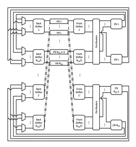
Figure 4.6: Block diagram of general overall decoder with fully parallel VNs and CNs possibly parallelized;  $N_{VN}$  and  $N_{CN}$  are the total number of hardware VNs and CNs, respectively.
