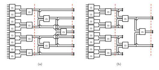
Figure 4.4: Check nodes that : (a) do not have and (b) have the variable depth pipeline; the dashed line indicates a register and the arrow indicates an output.
