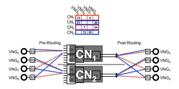
Figure 5.15: Illustration of pre- and post-routing for a section of the rate 1/2 matrix.
