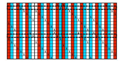
Figure 4.8: Example of why decoder cannot have serialized VNs and non-fully layer serialized CNs.
