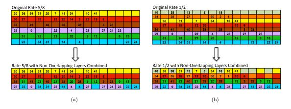
Figure 5.4: The four disjoint sets of non-overlapping layers for the (a) rate 5/8 and (b) rate 1/2 matrices.
