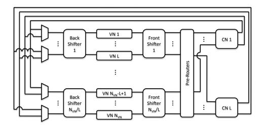
Figure 4.5: Block diagram of general overall decoder with CNs layer serialized and VNs possibly serialized;  $N_{VN}$  is the total number of hardware VNs.
