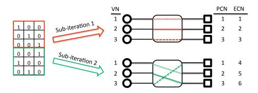
Figure 3.4: Simplified routing with AA matrices.
