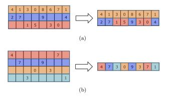
Figure 4.1: Examples of compressing matrices with : (a) two non-overlapping layers ; (b) four non-overlapping layers.
