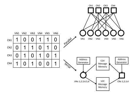
Figure 3.1: Fully parallel and fully serial architectures for the same LDPC matrix.
