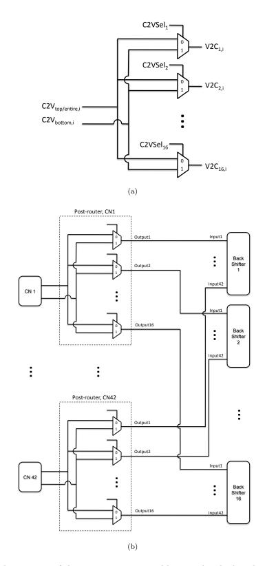
Figure 5.18: Implementation of the post-routers required by granular check nodes : (a) post-router structure for CN i; (b) routing between CNs, post-routers, and back barrel shifters.
