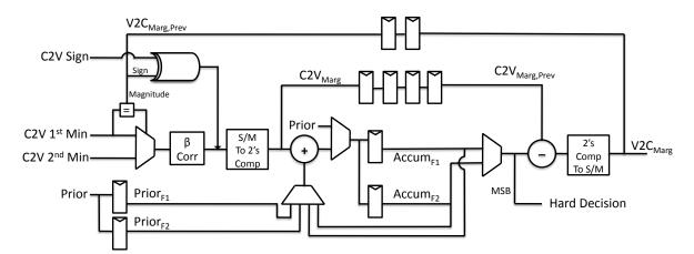
Figure 5.11: Variable node architecture.
