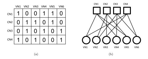
Figure 2.1: LDPC code example: (a) parity check matrix representation, (b) Tanner graph representation.
