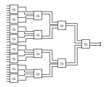
Figure 4.2: Standard check node architecture consisting of a tree of compare-select (CS) blocks.
