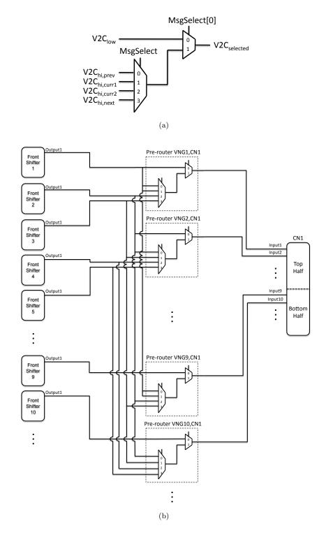
Figure 5.17: Implementation of the pre-routers required by granular check nodes : (a) structure of individual pre-routers; (b) routing between front barrel shifters, pre-routers, and CNs.
