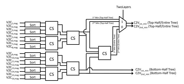
Figure 5.12: Check to variable message magnitude computation.
