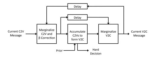
Figure 4.7: Variable node block diagram.
