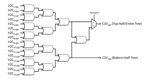
Figure 5.14: Check to variable message sign computation.
