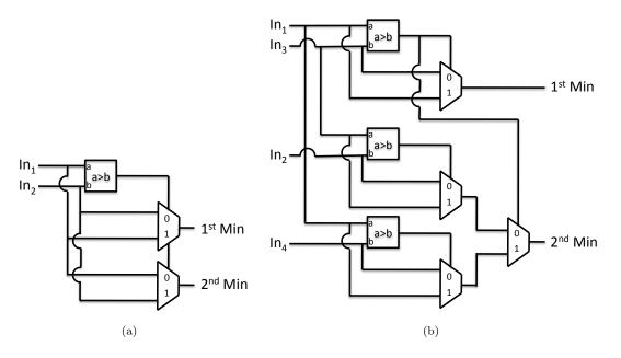
Figure 5.13: Structure of check node building blocks : (a) sort; (b) compare-select.
