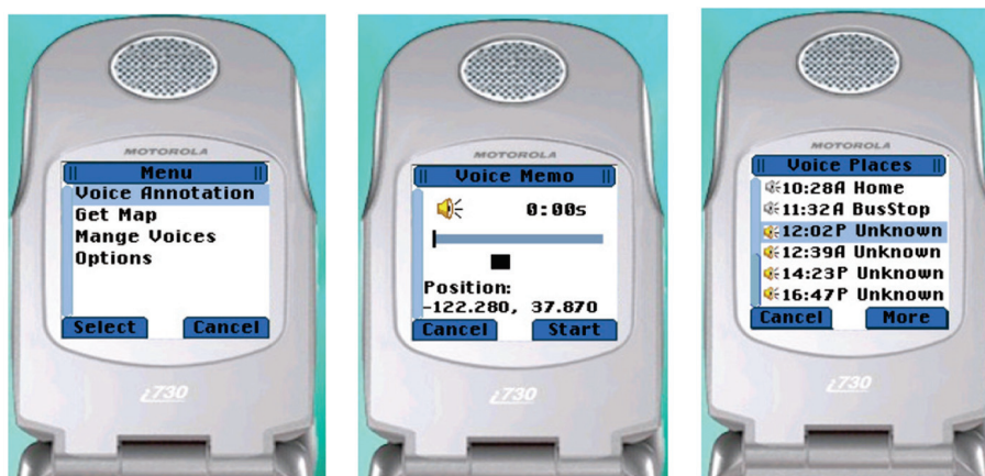
Figure 5.8: Cell phone interfaces for Voice . 5.8.1 Initial interface after activation. 5.8.2 voice capture interface, 5.8.3 voice history. After pressing the ok button in 5.8.3, the DText interface will pop up.
