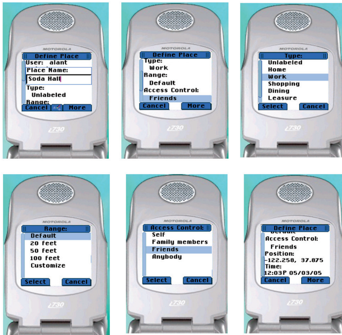
Figure 5.5: Cell phone Interfaces for DText . (number order is left to right, top to bottom) figure 5.5.1 represents the upper part of the primary menu. 5.5.2 represents the middle part. 5.5.3 is the place type collection sub-menu. 5.5.4 is the place range collection sub-menu. 5.5.5 is access control sub-menu. 5.5.6 is the bottom part of the primary menu.
