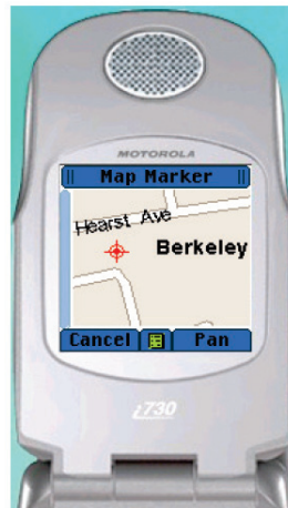
Figure 5.6: Cell phone interfaces for Map . After pressing the ok button, the DText interface will pop up for place annotation collection.
