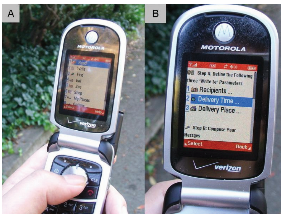
Figure 5.1: The GLAZE client running on a Motorola v325 cell phone. A. main menu. B. top part of the “write-to” primitive definition template.
