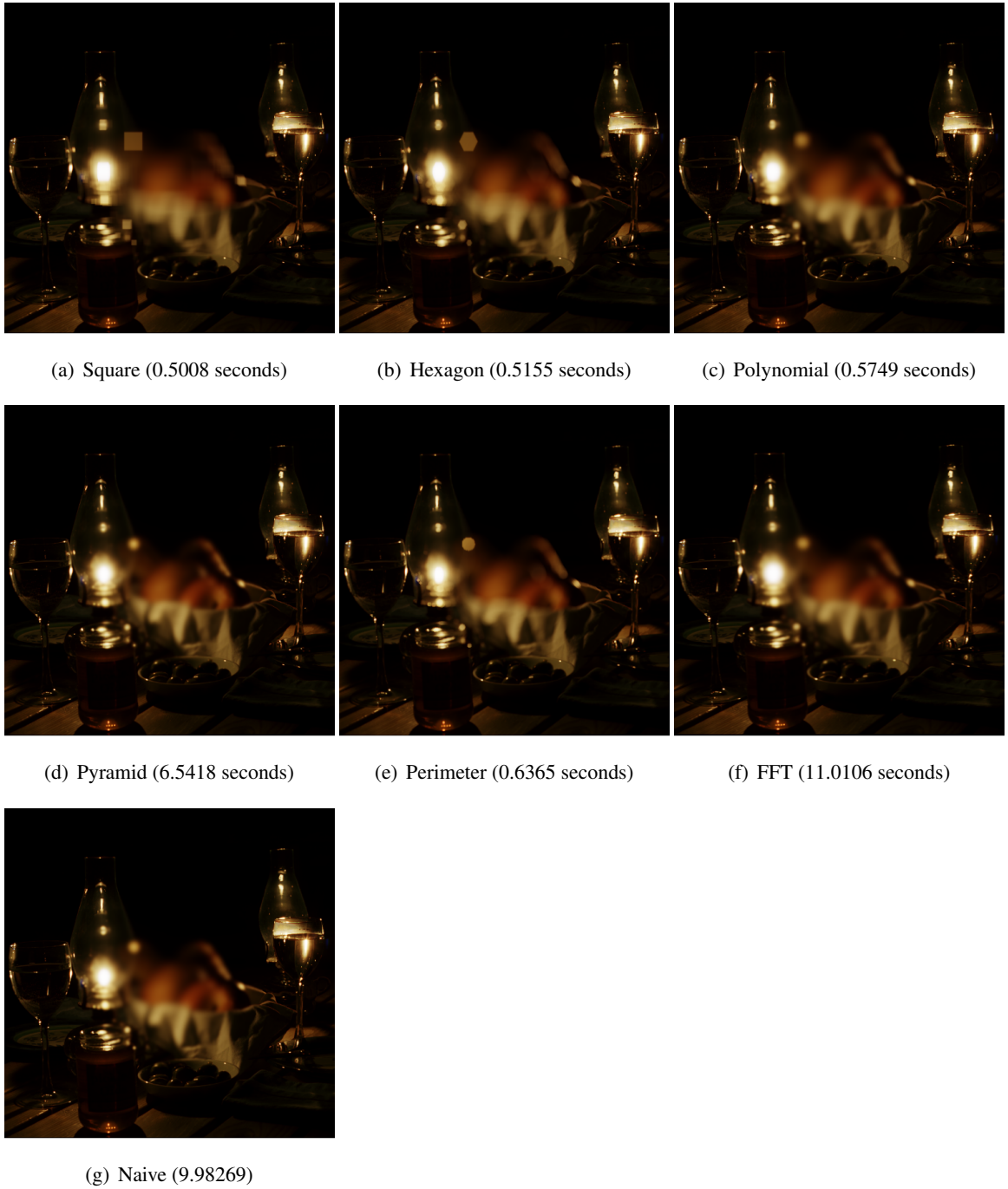
Figure 8.4: Various blur methods used on a high dynamic range image. Observe that the methods produce significantly different results.
