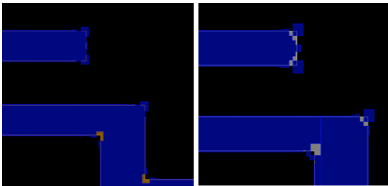
Figure 4.10: Layout features under the two OPC treatments—‘mild’ OPC with smaller and fewer edges and ripples, and ‘aggressive’ OPC with more edges, larger edges and more iterations.
