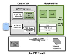
**Figure 1**—PTT System Architecture. The protected VM is emulated via QEMU in the control VM when it accesses tainted data. The PTT-ext3 filesystem is located in the control domain and the protected VM communicates with it via a shared memory RPC mechanism.
