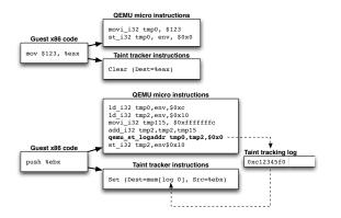
Figure 2—Example of QEMU code translation for emulation and taint tracking.
