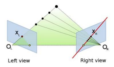
Figure 5: The point  $X_L$  observed in the left image must be observed in the right image along an epipolar line shown in red.  $O_L$  and  $O_L$  denote the focal points of the left and right image respectively.
