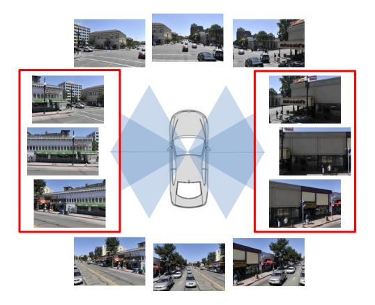
Figure 7: 6 images are extracted from each vehicle capture location. Each image has a 60° field of view and are oriented at 60°, 90°, 120°, 240°, 270°, and 300° angles with respect to the front of the capture vehicle.
