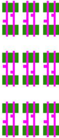
Figure 5.8: Second Layout Context for NAND2 Timing Characterization.
