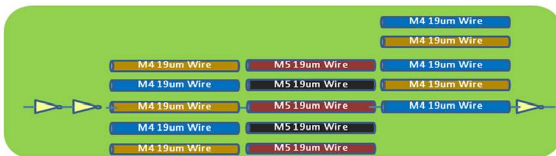
Figure 4.12: Three Segment Interconnect Structure #2
