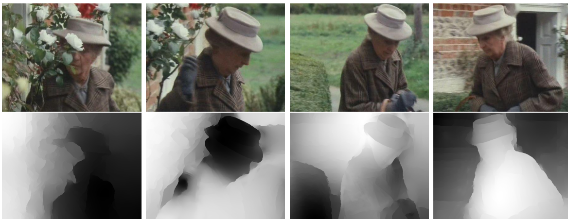
Figure 7.6: Illustration of “leakage” in eigenvectors for long range video sequences. This sequence is one of the sequences in the Motion Segmentation data set [35] and is a scene from the movie “Miss Marple : Murder at the vicarage”. Top Frames 1, 65, 120, 200 from the sequence. Bottom Corresponding portions of the second eigenvector. The vectors are normalized independently for better visualization. However, note the scale difference in the eigenvectors for each of the frames [0.899, 1.00] , [0.430, 0.941] , [0.156, 0.293] , [0.004, 0.066] .
