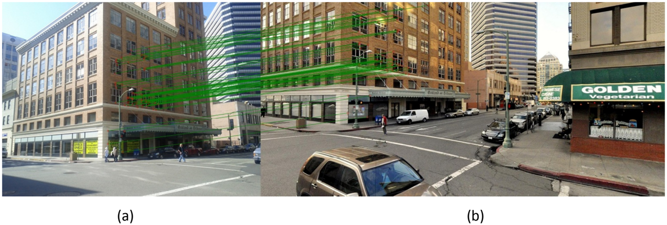
Figure 8: An image showing the feature correspondence inliers for the solution set, with lines connecting the point features on (a) the query image which match with those on (b) the database image.
