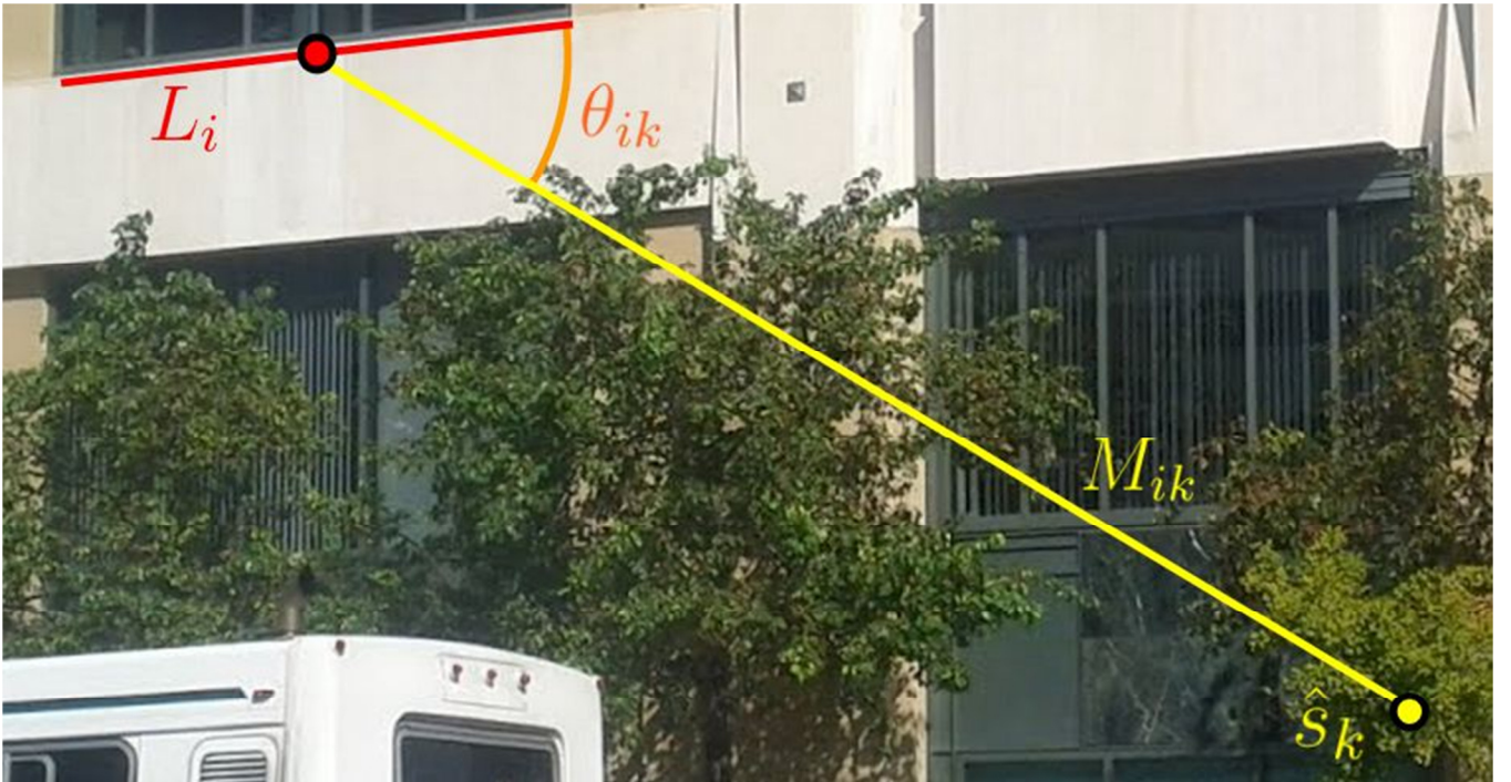
Figure 4: An example image line, vanishing point seed, and the pair's associated seed angle error.
