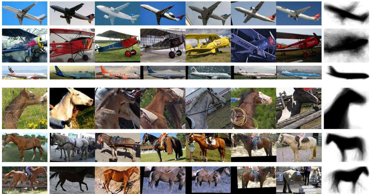
Figure 5.5: Visualization of some of our components for aeroplane (top) and horse (bottom) categories. Each row corresponds to a component. The left-most images are seeds; the middle six images are top aligned objects for each seed; and the right-most images are averaged mask of top 32 aligned objects. Note that, by design, objects within each component are tight in configuration space.
