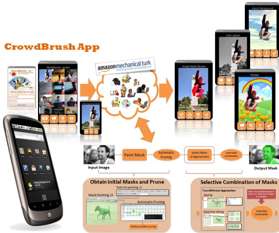
Figure 2: System design overview of crowdsourced rotoscoping system, including a client-side mobile application on Android (upper half) and a server-side automated pipeline for crowdsourcing (bottom half)
