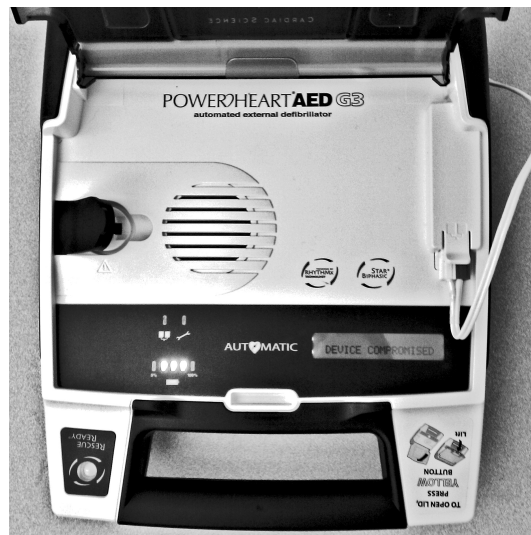
Figure 4.1: The Cardiac Science G3 Plus exploited to install our custom firmware. The AED displays DEVICE COMPROMISED.
