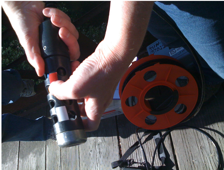
Figure 5.1: Expensive (approximately $2,000 per unit) but accurate water testing equipment used by a local watershed group to test water quality. The probe is being placed into its protective casing after calibration by the volunteer. The error-prone reel of wiring which connects this probe to the monitoring unit is visible in the background.
