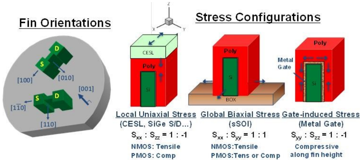
Figure 3.4, Multiple-Gate FET design variations: \langle 100 \rangle and \langle 110 \rangle fin orientations (left) and under different stress configurations (right).
