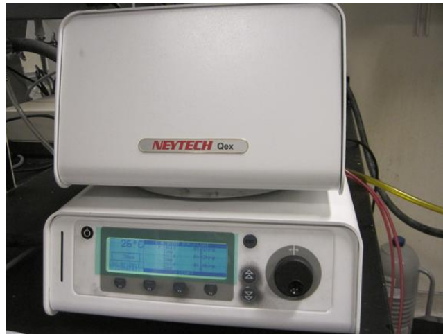
Figure 86. Centurion NeytechQex vacuum furnace used for thermal bonding of glass wafers.
