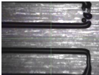
Figure 43. Inaccurate landing of drops in a pattern due to increased print height.
