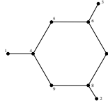
Figure 4.15: IEEE 9-bus benchmark network. Bus 1,2,3 are generators and the rest of the buses are loads.
